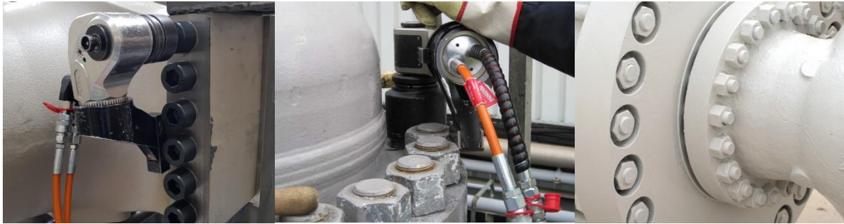
Actuation of shut-off valves with the MSX hydraulic torque wrench
