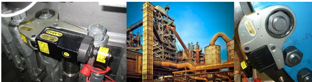
The hydraulic cassette tool FSX for pipe flange and gate valve connections for a tandem application of a blast furnace end flange connection
